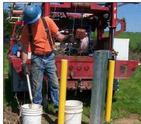
Water being drawn from a monitoring well.
